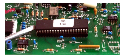
Fig. 8, 9: Gently pry the old chip out by lifting on alternate sides of the socket with a small screwdriver.
