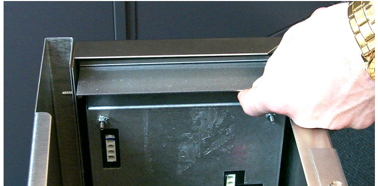
Fig.13: Position the deflector shroud on the upper mounting studs of the computer assembly.
